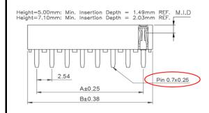
Insulator Height = 5.0mm. Min. Insertion Depth = 1.49mm Insulator Height = 7.1mm: Min. Insertion Depth = 2.03mm
